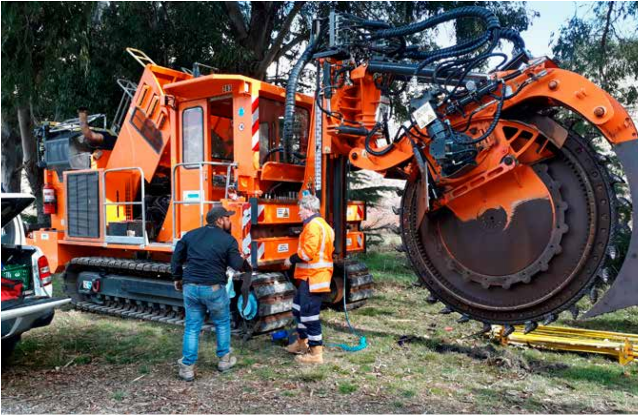
25-tonne rock saw for use on the fibre link projects
