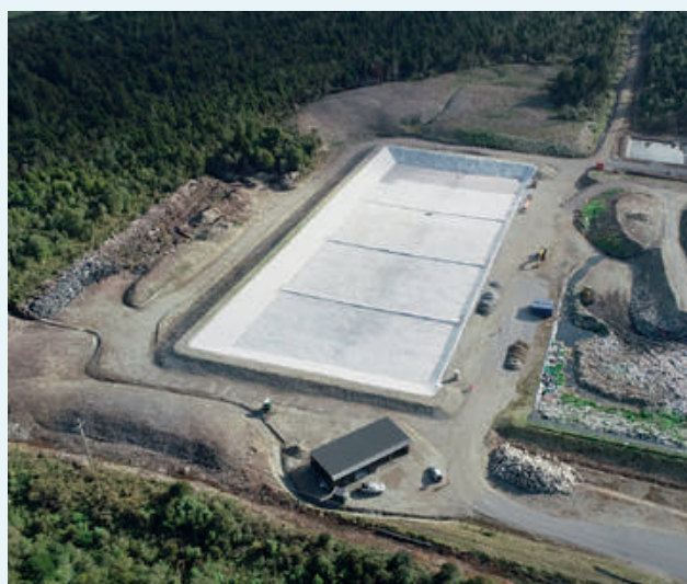
Butlers Landfill, West Coast – Lining new cell
