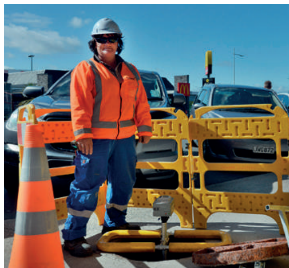
Sewer Line Rapid Assessment Tool (SL-Rat) in action in Taupō CBD.
